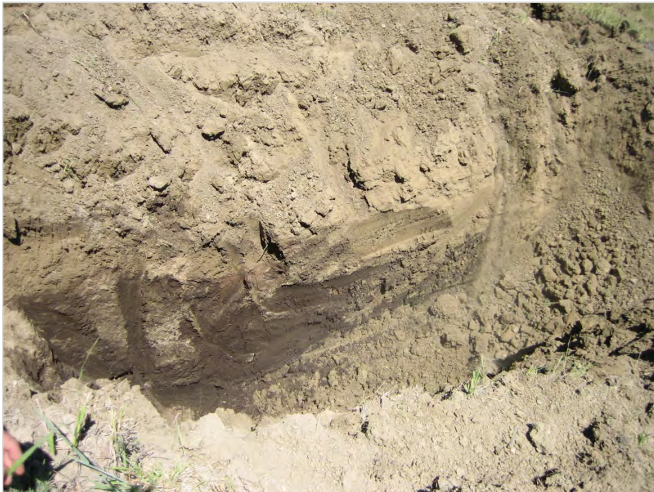
Photograph 2: Organic laden soils below surface clays
