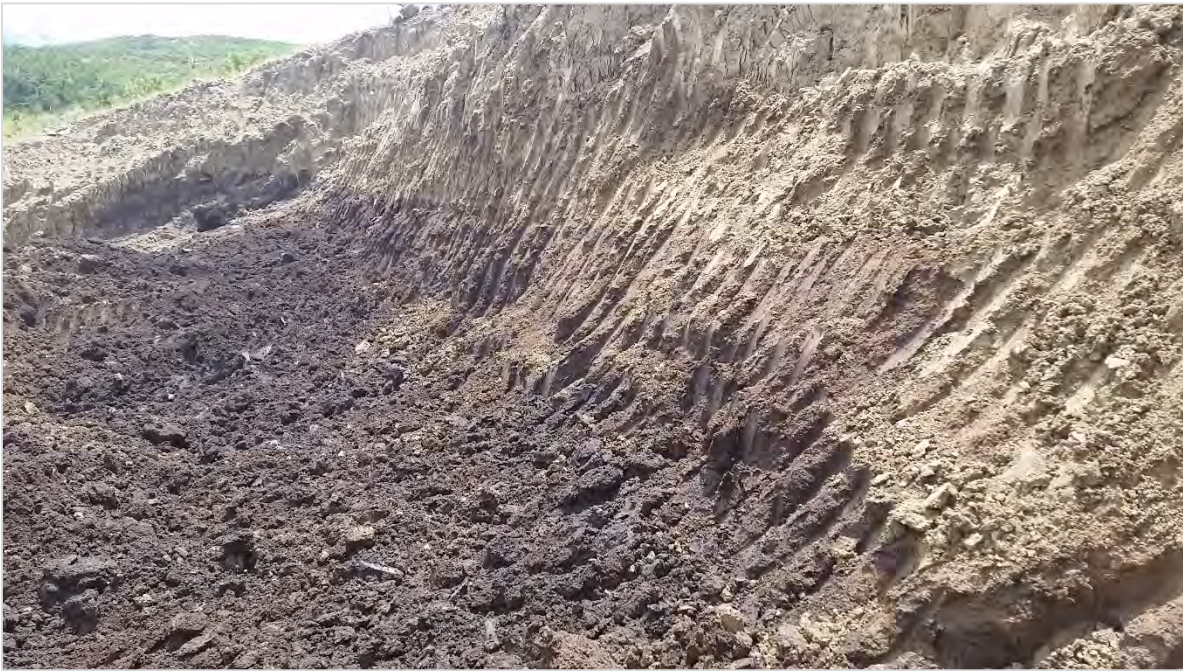
Photograph 16 showing the nearly constant elevation of the organic material in the north cut face which seems to indicate that the organics are along a former dam crest elevation.
