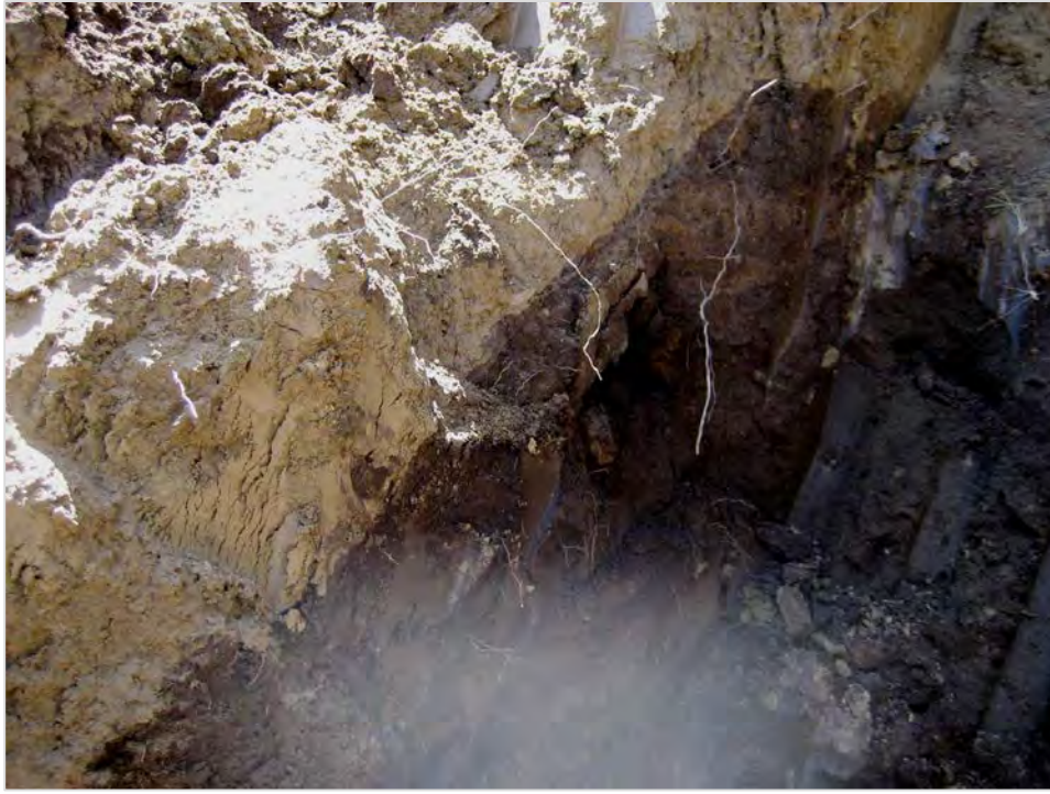
Photograph 1: Shows obvious contrast between clay embankment and organics at scarp slump area near top of test trench
