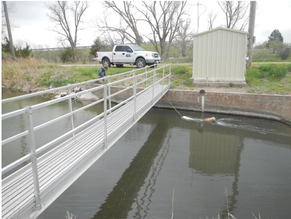
3. Manta 2 sonde deployment in the Kearney Canal downstream of the diversion.
