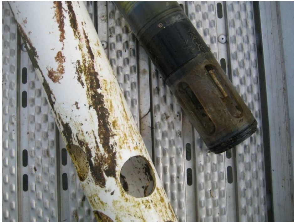
9. Biofouling of the Manta 2 deployed in the Kearney Canal downstream of the diversion near Elm Creek, NE.
