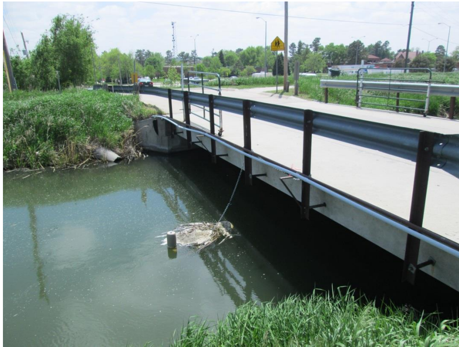
7. Biofouling of the Manta 2 deployed upstream of the Kearney Canal Hydro.
