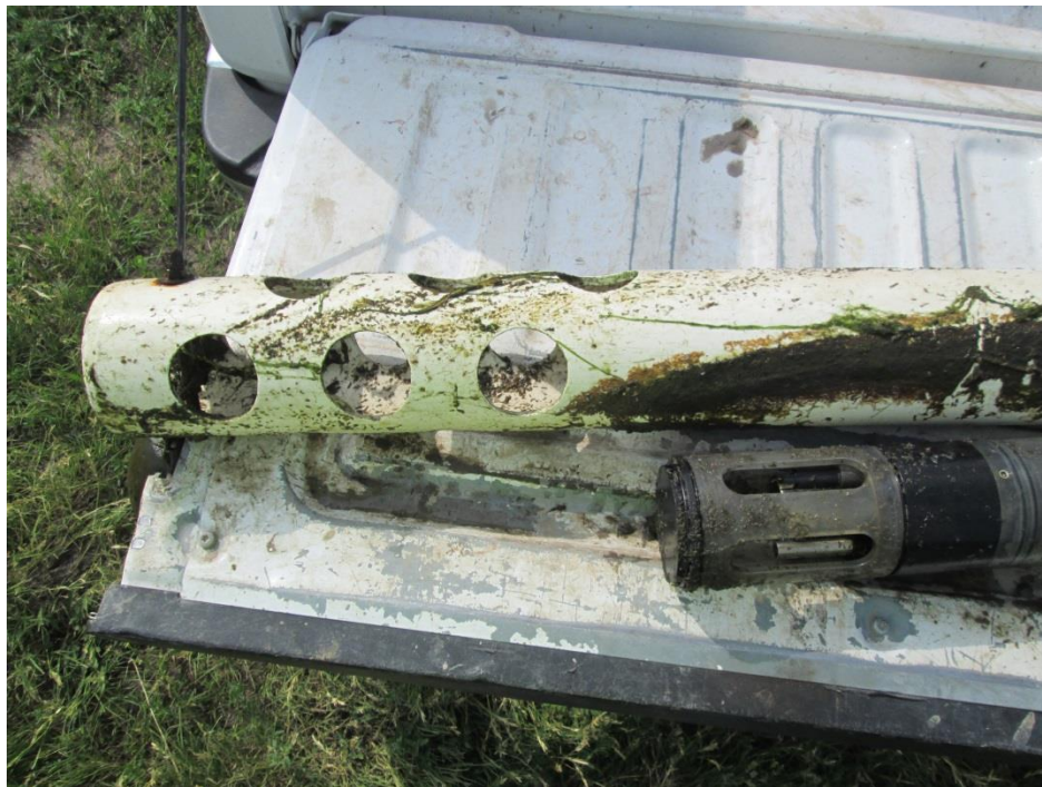
8. Biofouling of the Manta 2 deployed in the Platte River at Elm Creek, NE.
