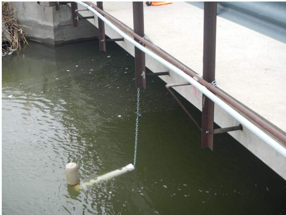
4. Manta 2 sonde deployment upstream of the Kearney Canal Hydro.
