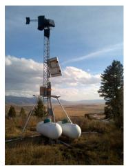
Also pictured at right is a white remote sensing unit called a radiometer. It takes vertical columns of atmospheric information that is similar to weather balloons but is continuous data. They are portable,
