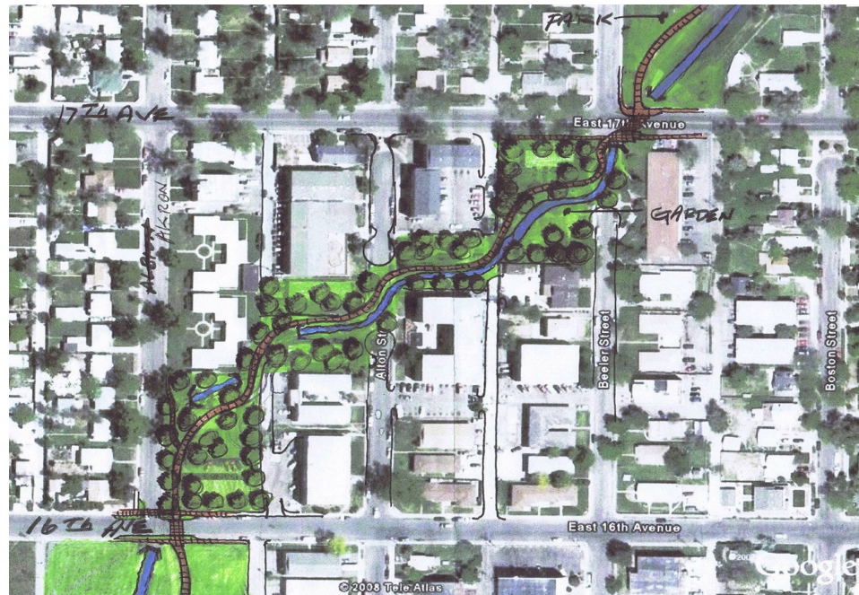
Figure 5.22 - Conceptual Sketch of UDFCD Daylighted Channel From 16th Avenue to 17th Avenue
