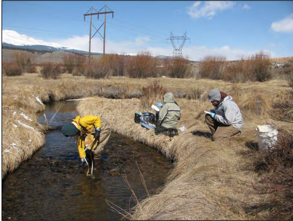
Figure 9. Reclamation Site Monitoring class completing Wolman Pebble count and water quality sampling.
