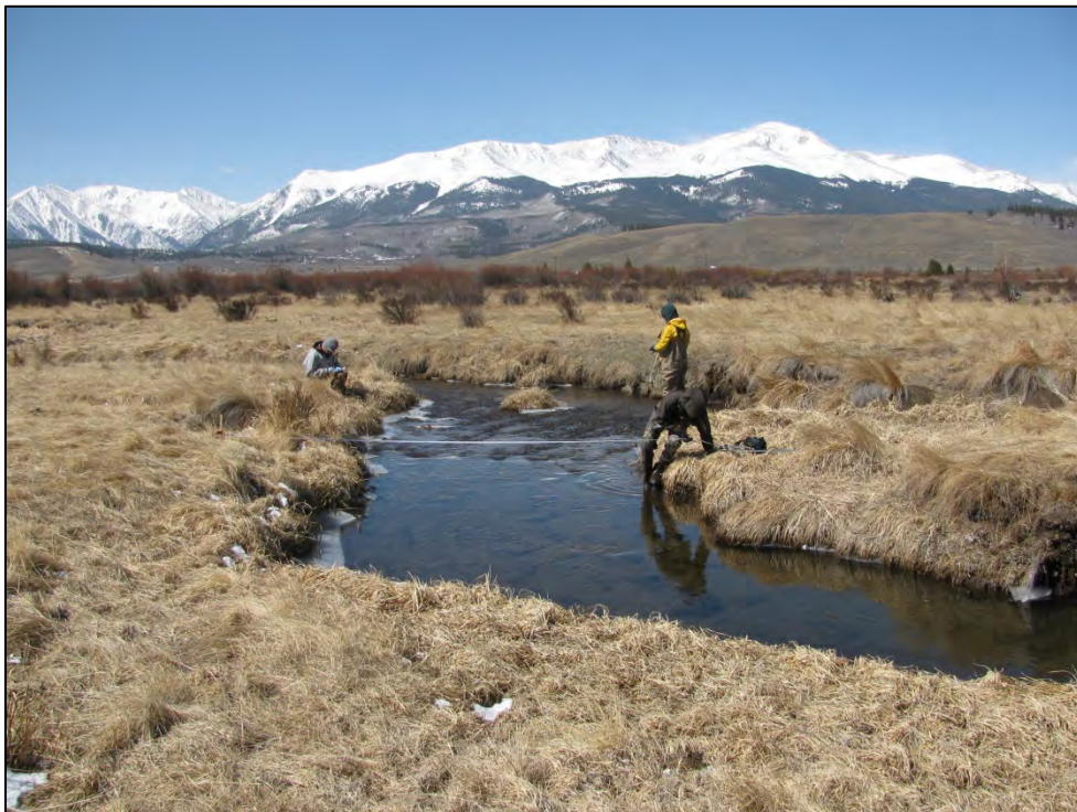
Figure 10. Reclamation Site Monitoring class conducting stream flow measurements.
