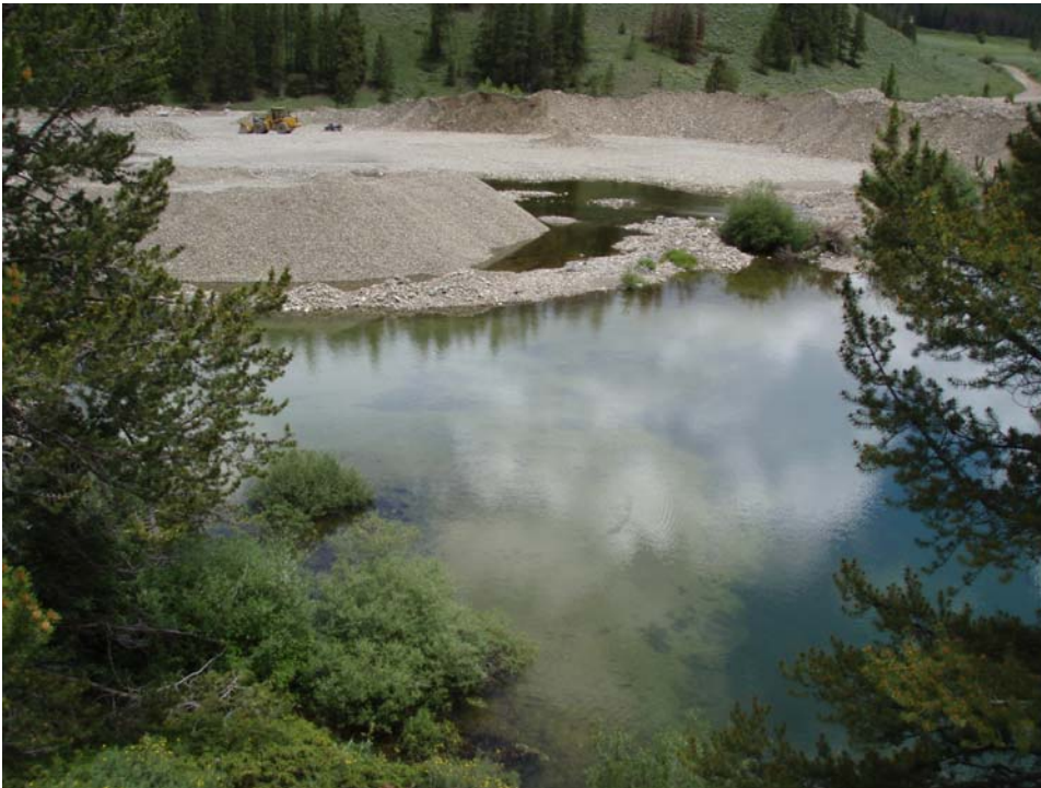
Photo 3 shows dredge piles and the on-going operation of removing the material. Standing water in the foreground is believed to be contact with the groundwater table.
