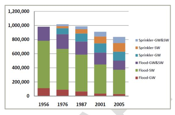
Figure 2-13. Water Division 1, Irrigated Acreage by Irrigation Type and Water Source
