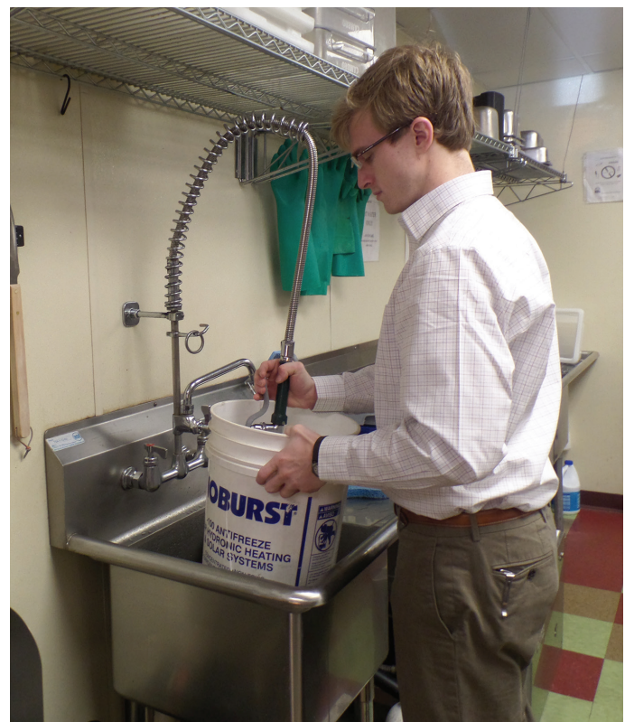
CRC auditor performs a flow test on a pre-rinse spray valve at Two Spoons Gelato Shop in Boulder.
