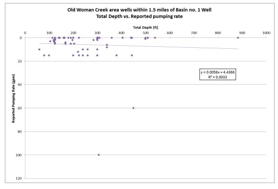
**Figure 8.9.** Graph of reported pumping rate versus total depth for water wells in OWC area within 1.5 miles of the proposed First Liberty Basin #1 oil well.
