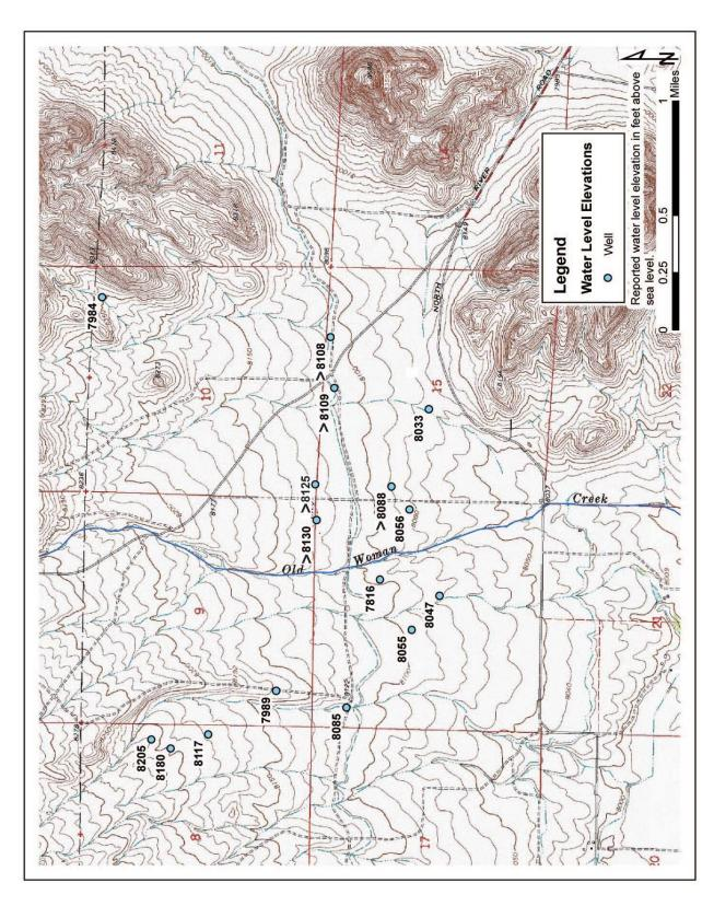
**Figure 8.12.** Map showing elevations of reported static water levels in OWC area. Flowing wells are marked by a "greater than" sign (>), which indicates water level is above that elevation.
