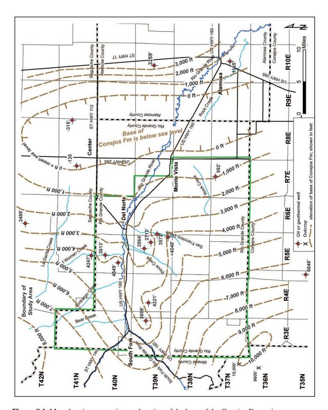
Figure 8.1. Map showing approximate elevation of the base of the Conejos Formation.
