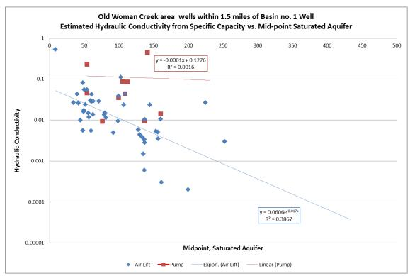
**Figure 8.11.** Graph of calculated hydraulic conductivity versus depth to estimated midpoint of saturated aquifer for water wells in the OWC area within 1.5 miles of the proposed oil well.
