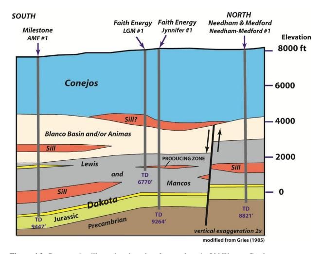
Figure 4.2. Cross section illustrating the subsurface geology in Old Woman Creek area.
