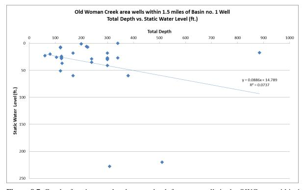
**Figure 8.7.** Graph of static water level versus depth for water wells in the OWC area within 1.5 miles of the proposed First Liberty Basin #1 oil well.
