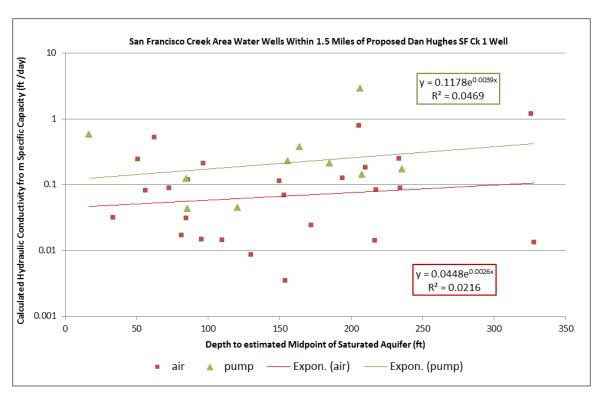
**Figure 8.10.** Graph of calculated hydraulic conductivity versus depth to estimated midpoint of saturated aquifer for water wells in the SFC area within 1.5 miles of the proposed oil well.
