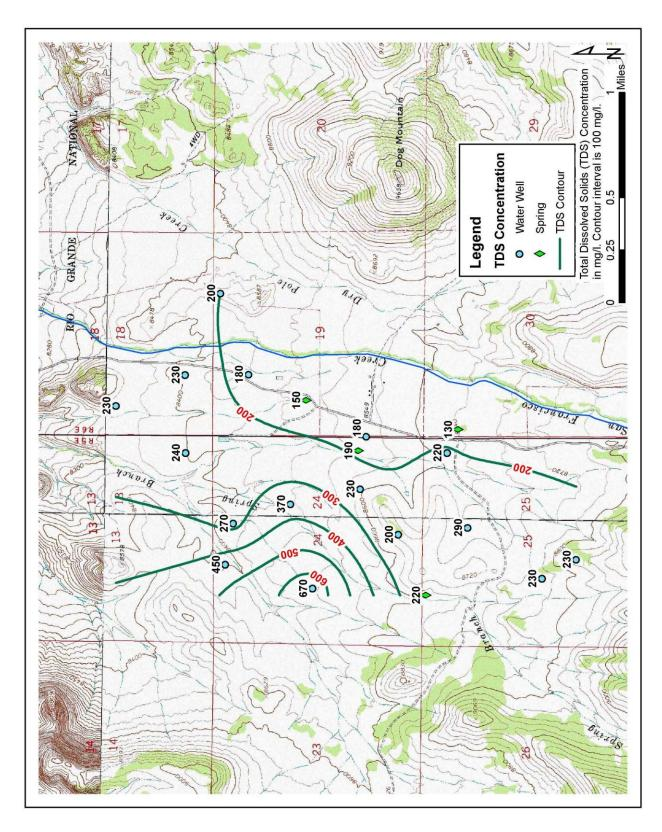
**Figure 6.11.** TDS (in mg/L) of well water and springs in the San Francisco Creek area. Contour interval 100 mg/L.
