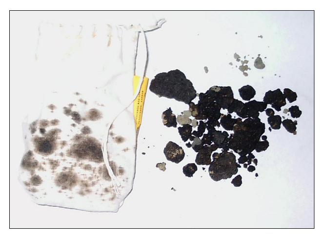
**Figure 7.2.** Photograph of oil-saturated cuttings from Falk water well. Note oil staining of cloth sample bag.
