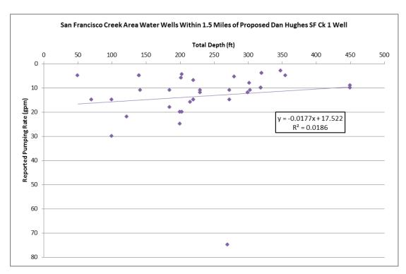
**Figure 8.8.** Graph of reported pumping rate versus total depth for water wells in SFC area within 1.5 miles of the proposed Hughes DAHC-San Francisco Creek #1 oil well.
