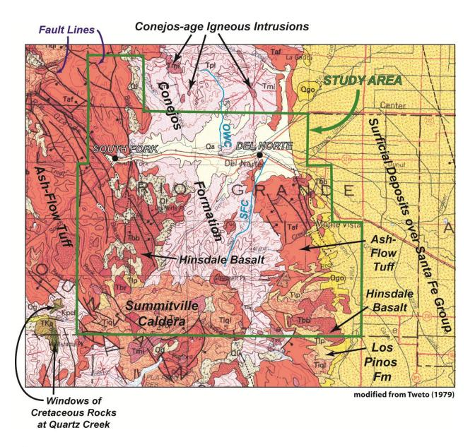
**Figure 3.3.** Simplified geologic map of the project area. Each geologic formation is shown in a different color, and the more important geologic formations are labeled with the large lettering. SFC = San Francisco Creek; OWC = Old Woman Creek. (modified from Tweto, 1979b)
