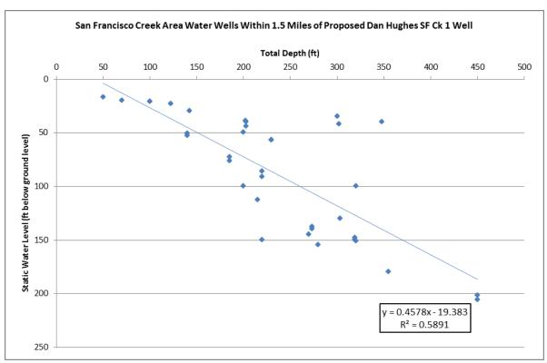
**Figure 8.6.** Graph of static water level versus depth for water wells in the SFC area within 1.5 miles of the proposed Hughes DAHC-San Francisco Creek #1 oil well.
