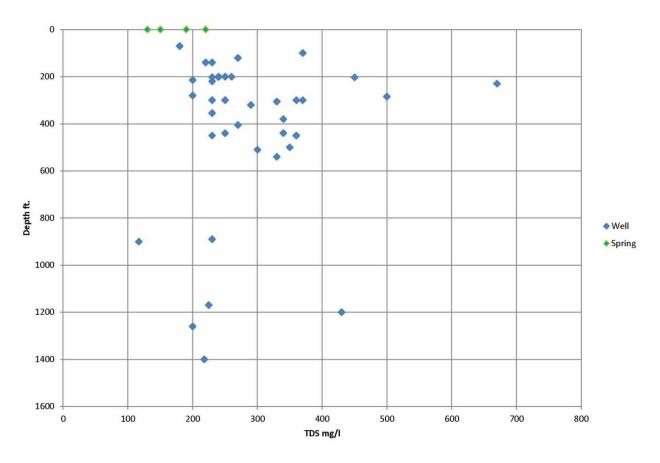
Figure 8.5. Graph of TDS versus depth for all water samples.
