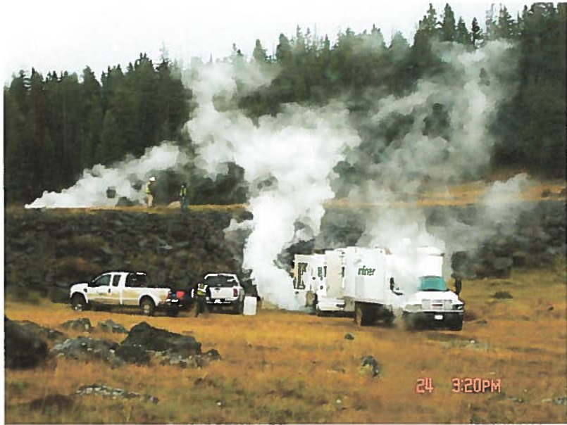
Figure 5 Steam being generated by the trucks.
