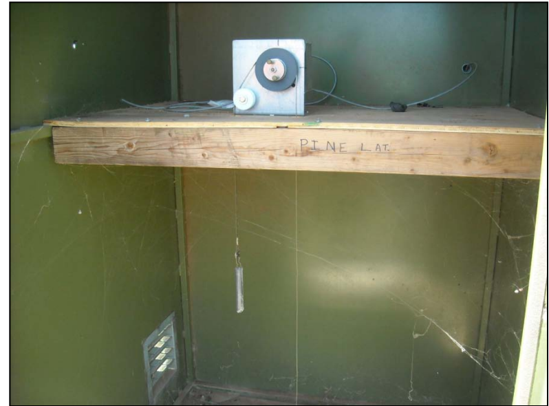
Photo 8: Pine lateral – measuring device – float level sensor.
