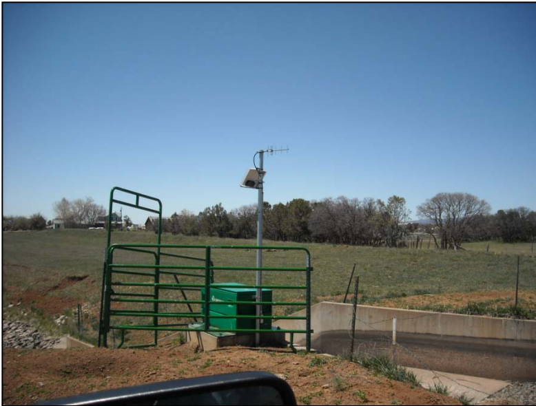
Photo 7: Florida Farmers Ditch West – level sensor housed in stilling well covered by utility box, including solar panel and antenna. Staff gauge also shown. Arrangement is typical of level sensor used along Florida Mesa canals.
