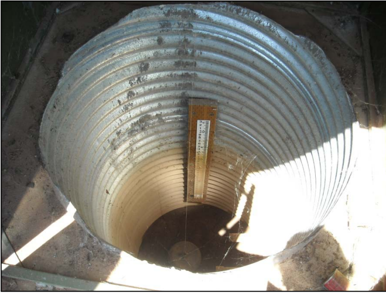
Photo 9: Pine lateral – Stilling well with staff gauge.
