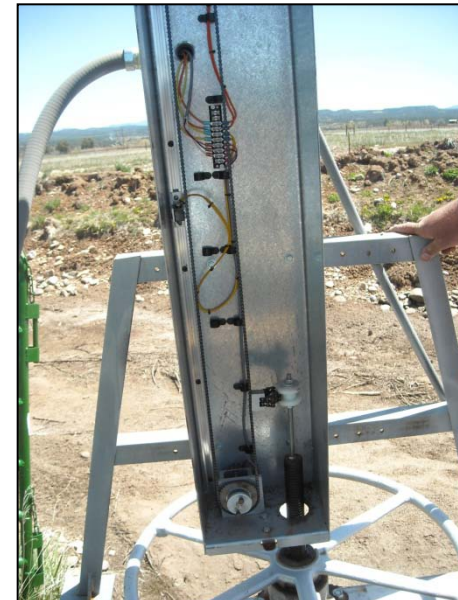
Photo 4: Florida Farmers Ditch West – Slide gate actuator.
