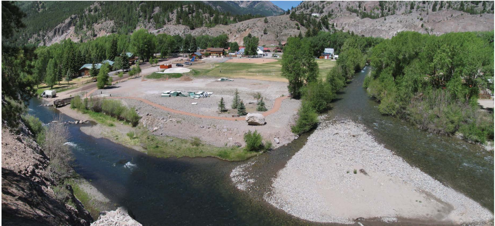
Figure 3. Photo of existing condition at confluence. Note large amount of gravel and cobble deposition.
