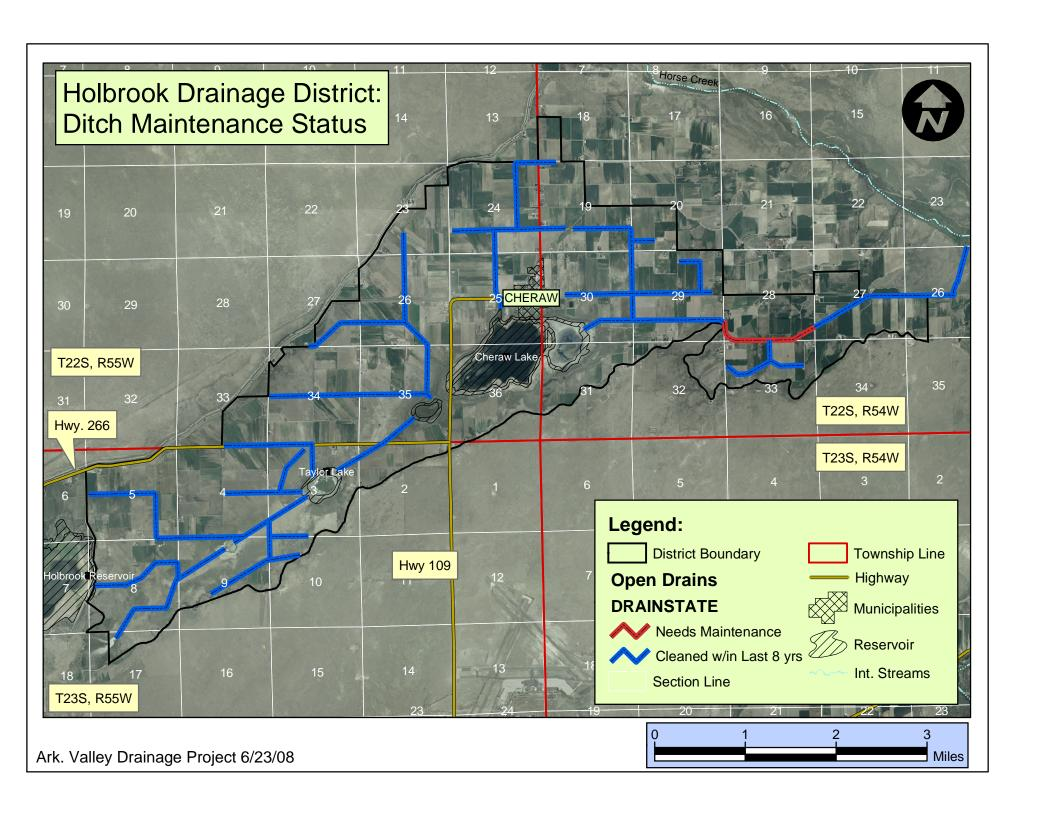
Drainage District Infrastructure notes on the Holbrook Drainage District located in Otero County, Colorado. This district includes all or parts of Sections 23 - 27, 33 - 36 of T22S, R55W, Sections 1 - 5, 8 - 10, 17 of T23S, R55W, and Sections 18 - 20, 26 - 35 of T22S, R54W.
