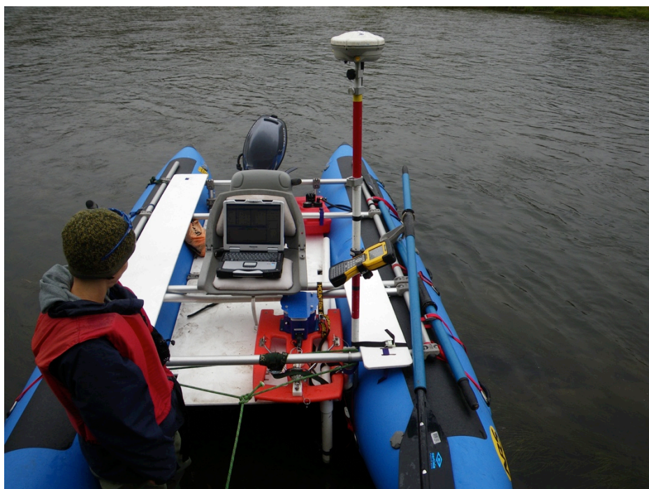
Figure 13. Setup of the ADCP, GPS rover unit, and laptop computer on a raft so that bed elevations and velocities can be measured.
