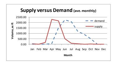
A similar chart is presented below representing the irrigation demands versus the reservoir supply or releases made from Summit Reservoir. Again, it should be noted that the reservoir supply is not sufficient to meet projected demands.
