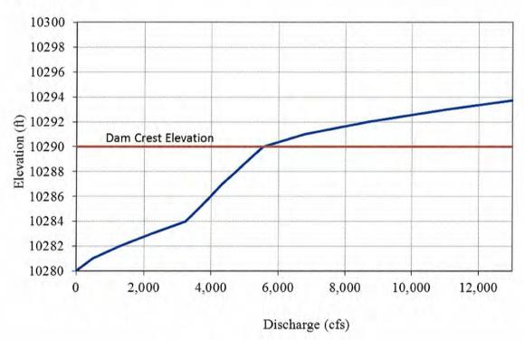
Figure 2-3 Discharge Rating Curve
