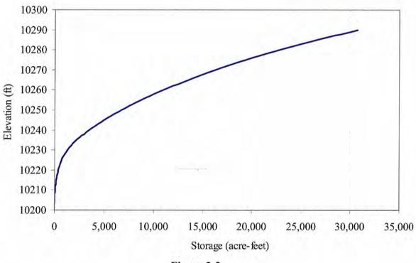
Figure 2-2 Storage Capacity Curve
