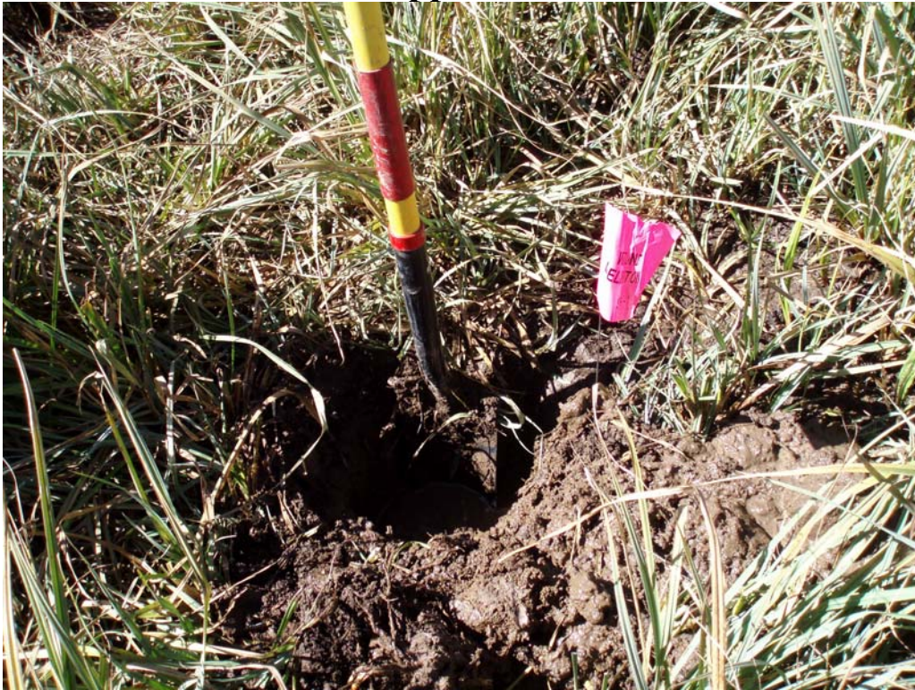
SP-1, typical of wetland fringe soils around entire Reservoir. Soil wetland indicators such as redox features were almost entirely lacking other than the presence of hydrology.
