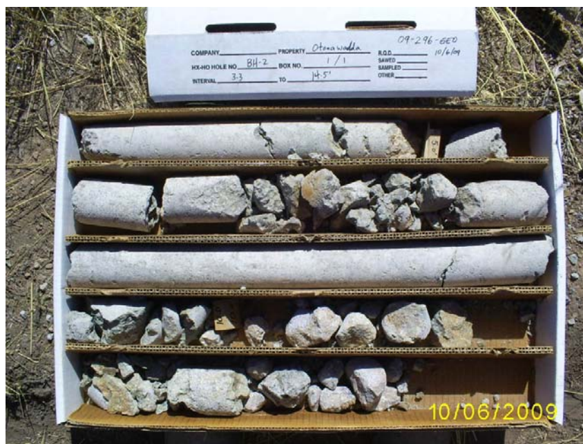
Recovered core from BH#2 (3.3-14.5 feet). The gravel-sized pieces of rock are indicative of highly fractured, and possibly more weathered bedrock zones.
