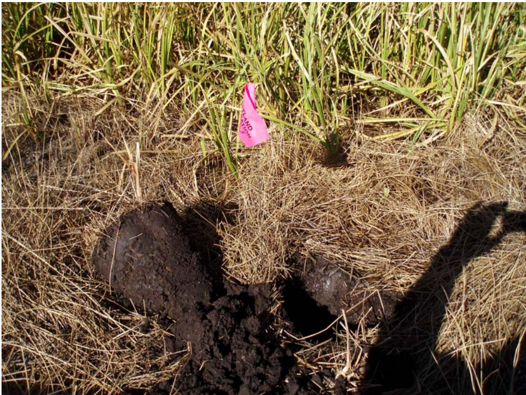
Study pit SP-3, typical of the wettest portions of the reservoir perimeter. Note lack of oxidized roots and other redox features.
