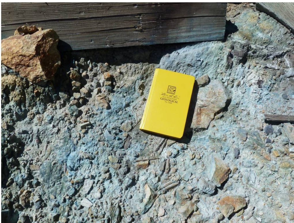
Photograph 15: Tailings from the Sill Mine Mill; note the blue-green color associated with copper salt precipitates and oxides.
