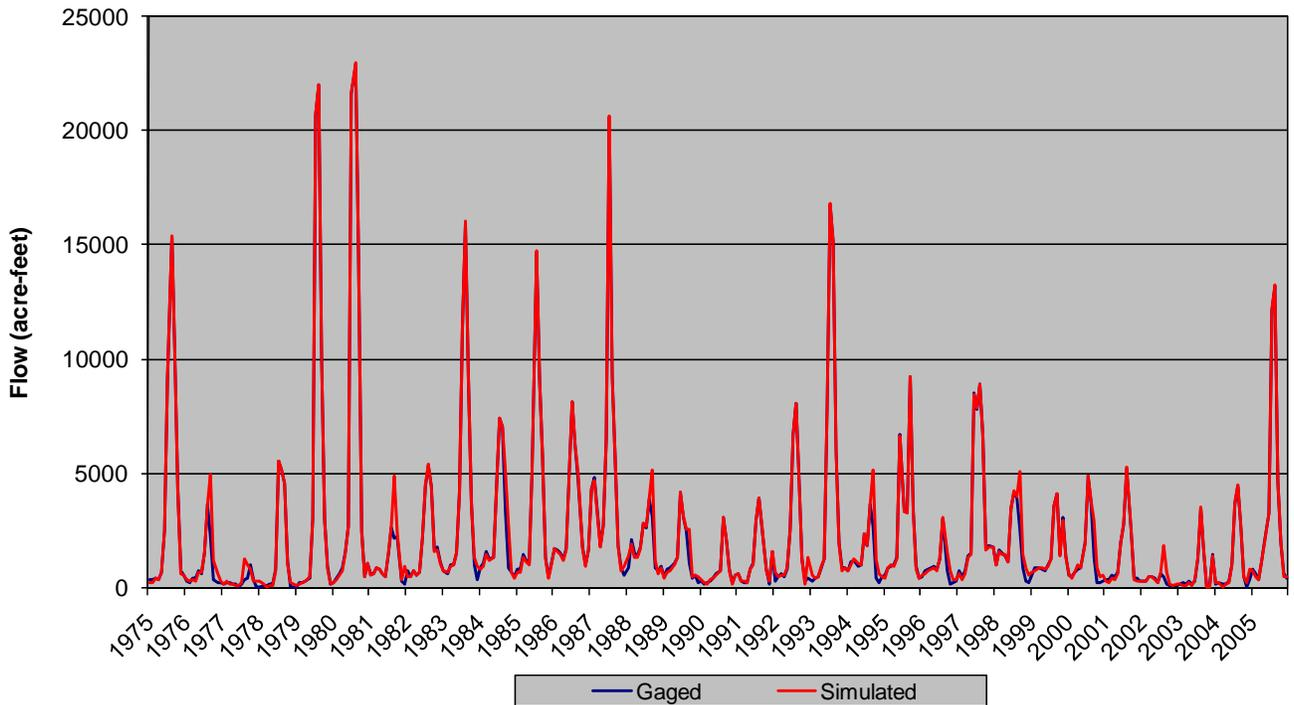
**Figure 7.6 Streamflow Calibration – La Plata River at Colorado-New Mexico Stateline**
