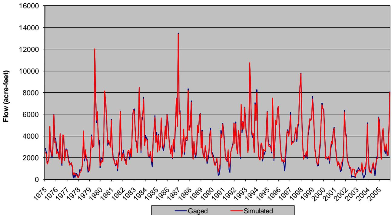
**Figure 7.8 Streamflow Calibration – McElmo Creek at Colorado-Utah Stateline**
