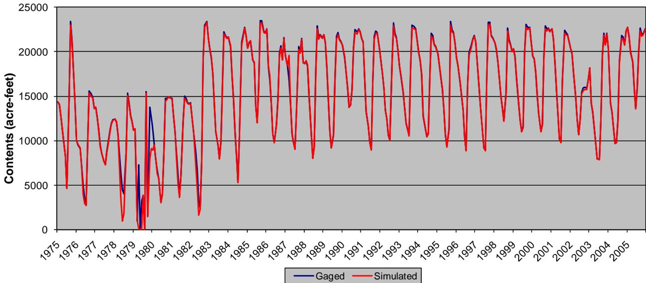
**Figure 7.13 Reservoir Calibration – Cascade Reservoir**
