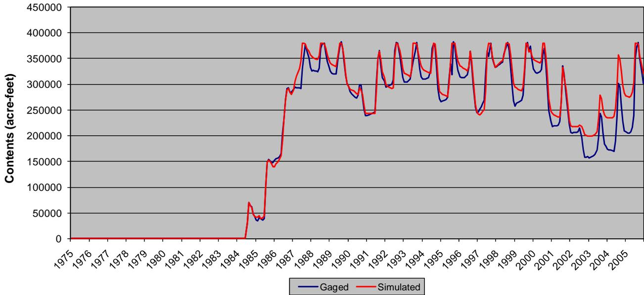
**Figure 7.15 Reservoir Calibration – McPhee Reservoir**
