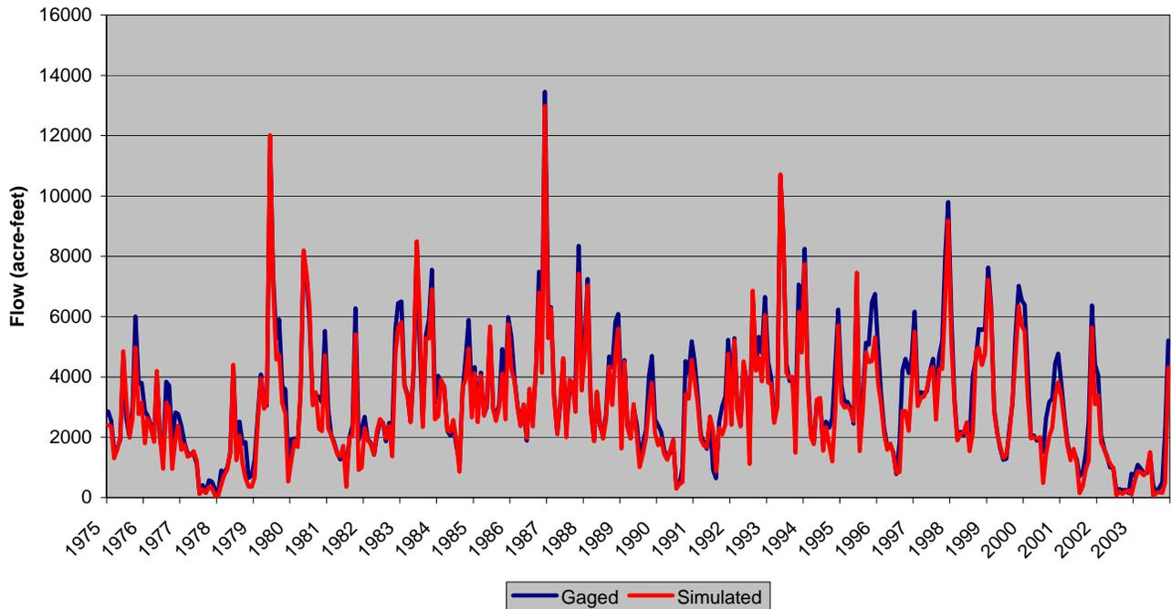
Figure D.8 Calculated Streamflow Simulation – McElmo Creek at Colorado-Utah Stateline
