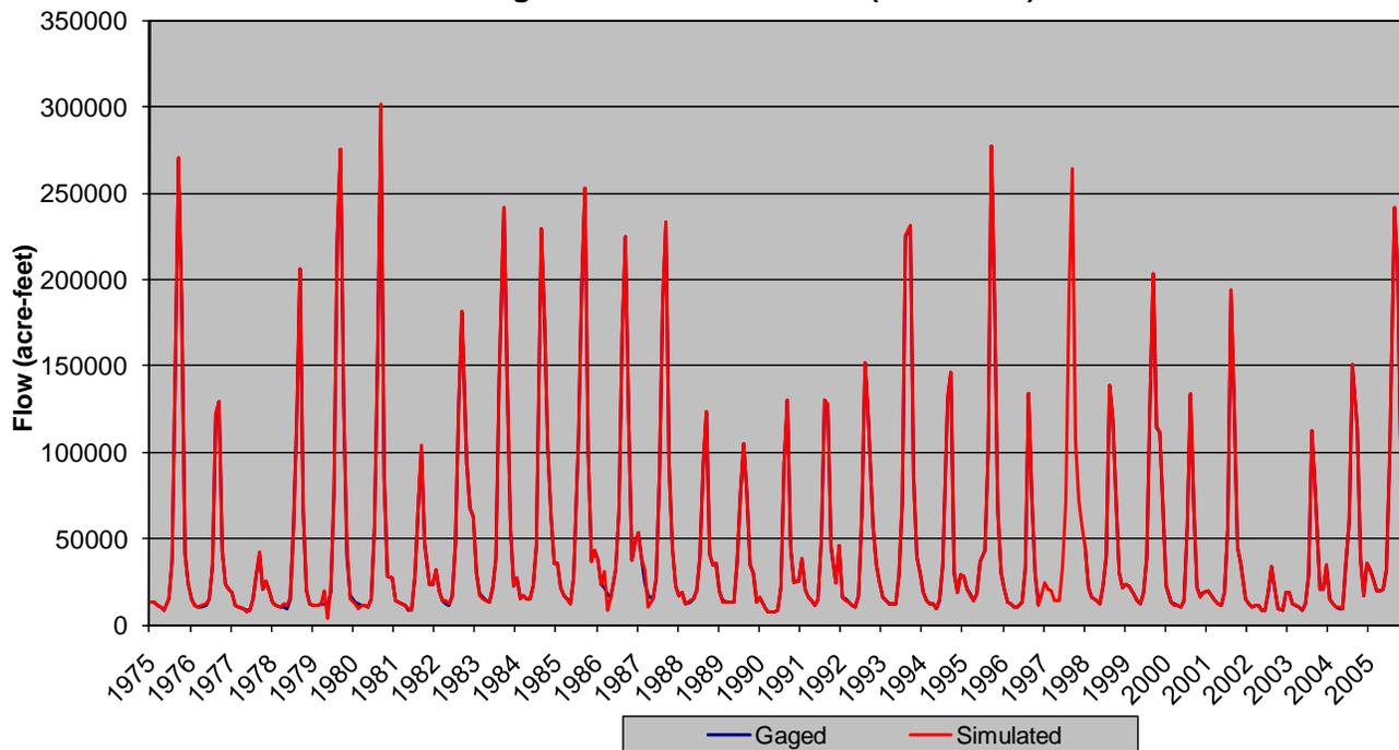
**Figure 7.5 Streamflow Calibration – Animas River at Durango**
