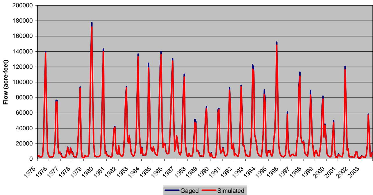
Figure D.1 Calculated Streamflow Simulation – San Juan River at Pagosa Springs
