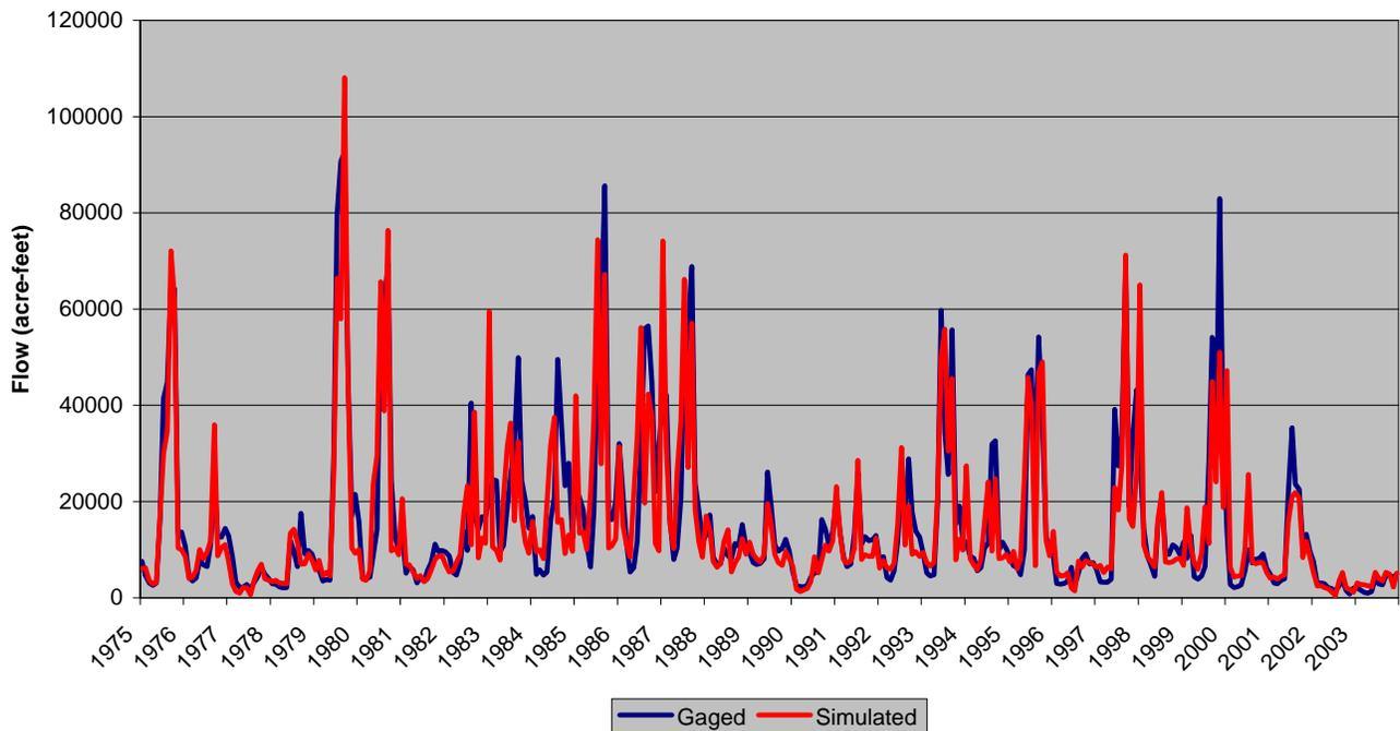
Figure D.4 Calculated Streamflow Simulation – Los Pinos River at La Boca
