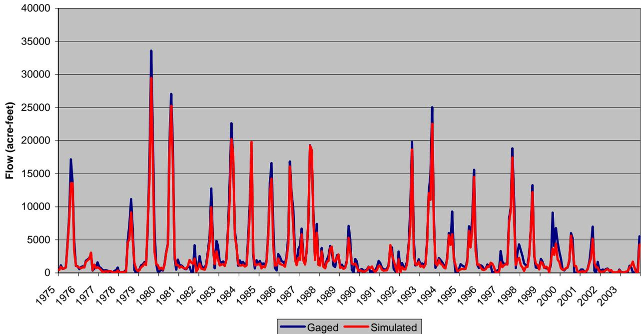
**Figure D.7 Calculated Streamflow Simulation – Mancos River near Towaoc**
