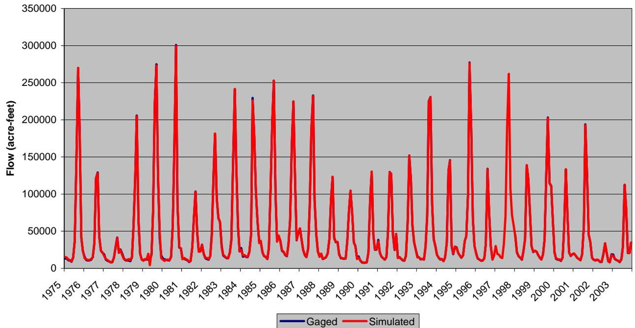
**Figure D.5 Calculated Streamflow Simulation – Animas River at Durango**
