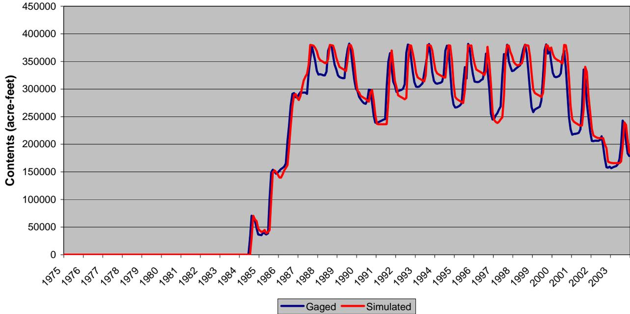
Figure D.15 Calculated Reservoir Simulation – McPhee Reservoir
