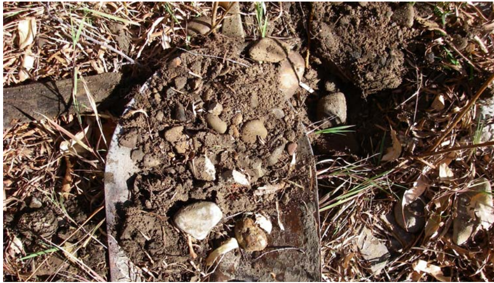
Photo 46. Brown flood plain materials (sand & sandstone) at Wildcat Canyon/Hwy 160 culvert.
