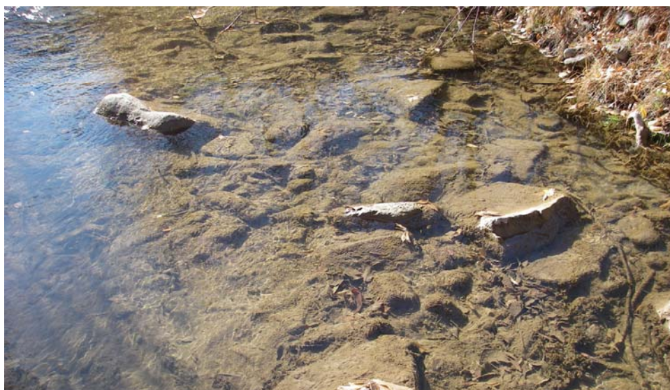
Photo 42. Channel bed with lots of fines at Wildcat Canyon – Lightner Creek confluence channel stability evaluation site.
