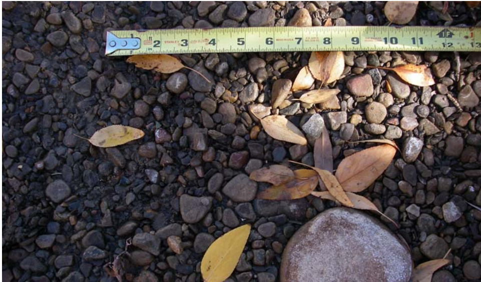
Photo 29. Bar composition ~ 100' upstream of Perins Canyon Road contains significantly less surficial shale material.
