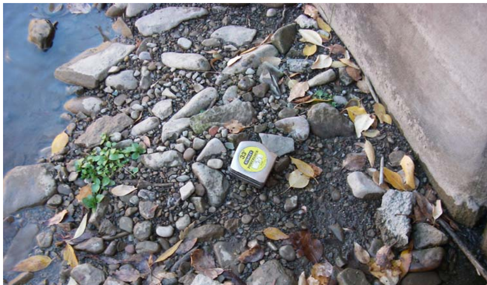
Photo 44. Depositional material at outlet of Wildcat Canyon/Hwy 160 culvert (no shale material apparent).
