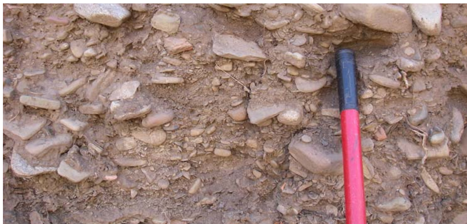
Photo 18. Close up of eroding colluvium bank south of Jiffy Lube.
