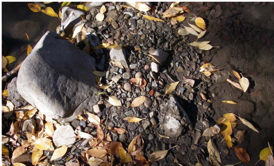
Photo 9. Typical bar material - shale (dominated by medium gravels and finer).
