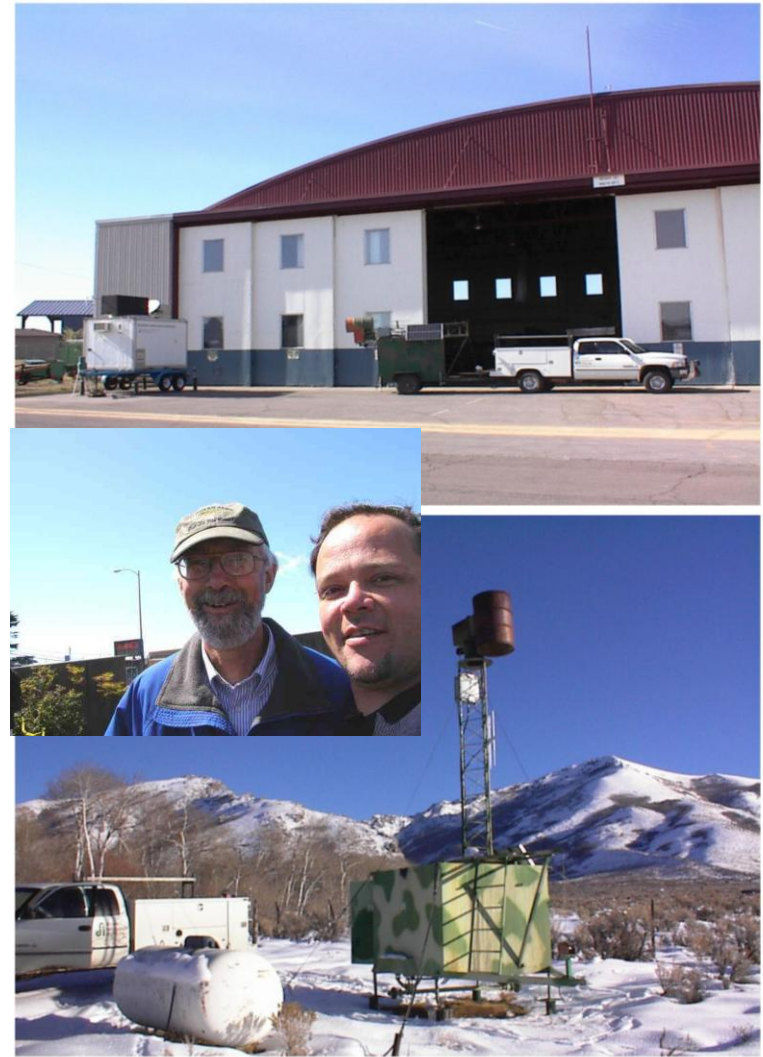
Figure 1. Top image shows a DRI generator ready for transport to a field site with tower assembly folded down onto the top of the trailer. Bottom image shows typical field installation with tower assembly raised and trailer wheels removed. Solar panel is just visible at the top right edge of the trailer and communications antenna is mounted about halfway up the right side of the tower. Seeding solution tank, nitrogen pressurization tanks, batteries and computer unit are housed inside the trailer.
