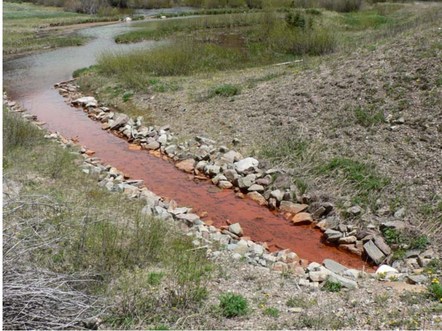
Photo 7.7. Ironoxide Deposits from the Silver Swan Point of Discharge into the Receiving Wetlands Area.
