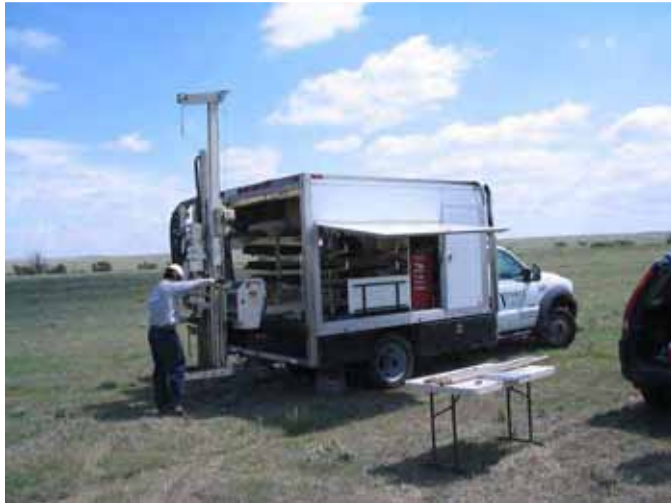
Geoprobe rig with soil sample table
