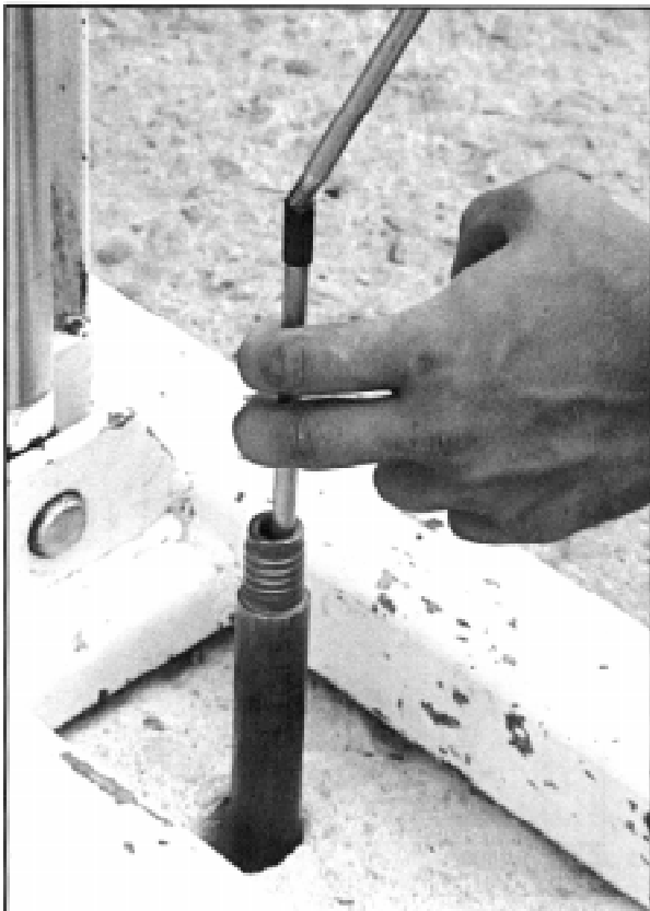
Figure 9. Coupling Extension Rods together.
