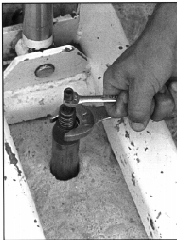
Figure 7. Tightening the Stop-pin.
