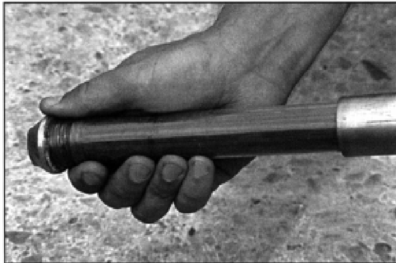
Figure 11. Removing the liner to recover the Sample.
